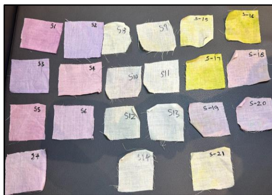
Fig. 1 Colour changes seen after pre-mordanting, simultaneous-mordanting and post-mordanting with pigments isolated from the plant waste material
