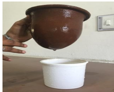
Fig 25: Water filtered from ceramic pot filter
