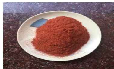
Fig 6: Saw dust used in making ceramic pot filter
