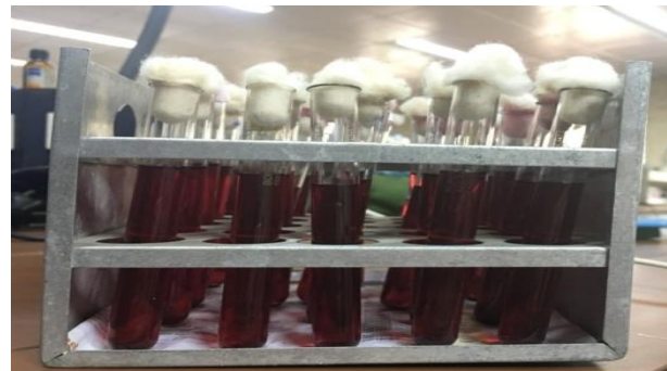
Fig 26: Preliminary test of treated water sample showing nil bacterial growth
