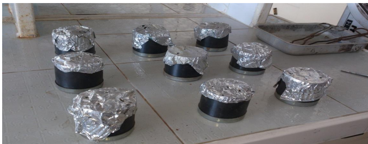
Figure (1): Peanut shells samples in metal cylinders intended for carbonization.
