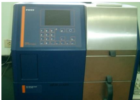
Figure 1. Grain and Flour Analyzer Infratec 1241
