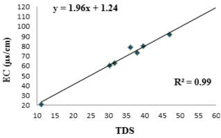
Fig.5. Linear regression of the average EC and TDS values in rainwater samples of the seven stations.
