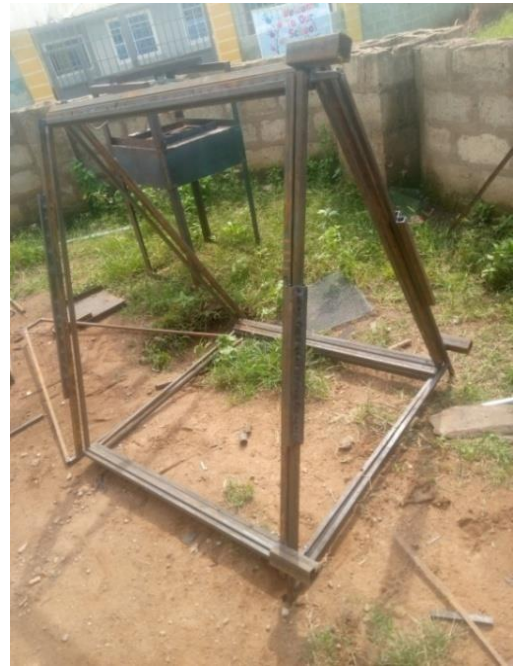
Plate 1b. Construction of a triangular ECS
