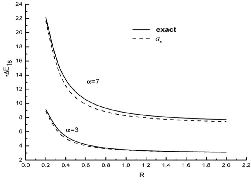
Fig.1. 1s - polaron shift with reduced QD radius  $R$  obtained by the approximation (15) (dashed line) and obtained by Green-function method [15] (solid line) for  $\alpha = 3$  and  $\alpha = 7$ .
