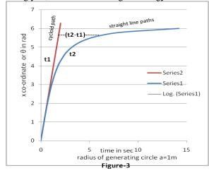
If the path of particle is restricted by wire or cycloid surface (any surface), we cannot avoid kinetic friction and air resistance. So I performed the experiment by taking cycloid of stainless steel surface and steel metallic ball of diameter 0.625 cm and mass 1.05 g. The maximum recoil vertical height gained by ball was 0.64 times original height. The energy lost by ball in first half cycle was 36%.
