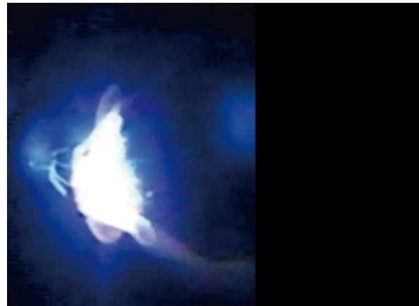
FIG 4 Photo of the arc discharge in a supersonic flow.
