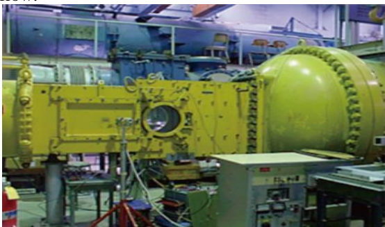
FIG 2 Mach 2.5 wind tunnel for performing the experiment
