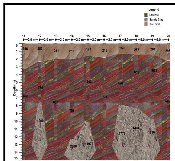
**Figure 5: 2D geologic section for shot points 11-20 station C and D, showing subsurface geology of the study area.**
