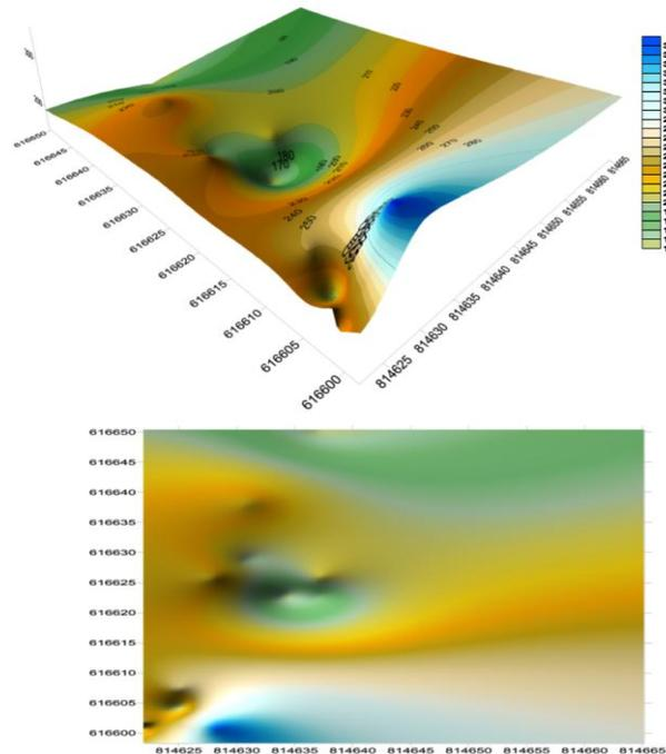
**Figure 6: (A) 3D Velocity model within layers 2 and 3 for shot points 6-20, computed from transformed velocities; (B) 2D view of the model. The model shows the geologic discontinuities (faults and fractures) in the subsurface.**
