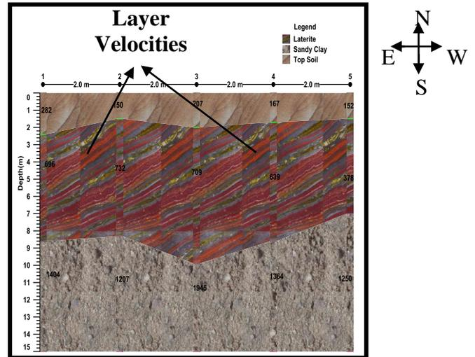
**Figure 3: 2D geologic section for shot points 1-5 station A, showing subsurface geology of the area.**
