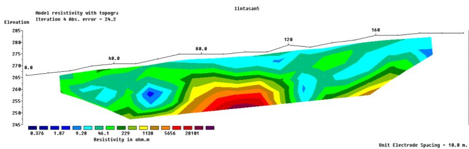
Figure 8: Subsurface resistivity 2D cross-section of line 5
