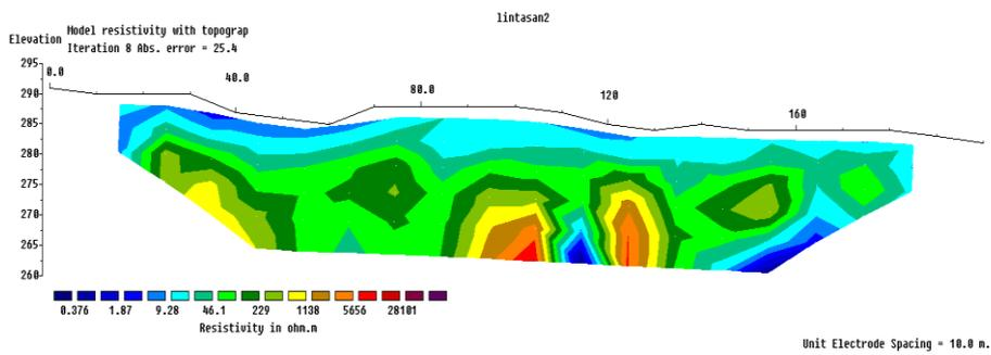
Fig 5: Subsurface resistivity 2D cross-section of line 2
