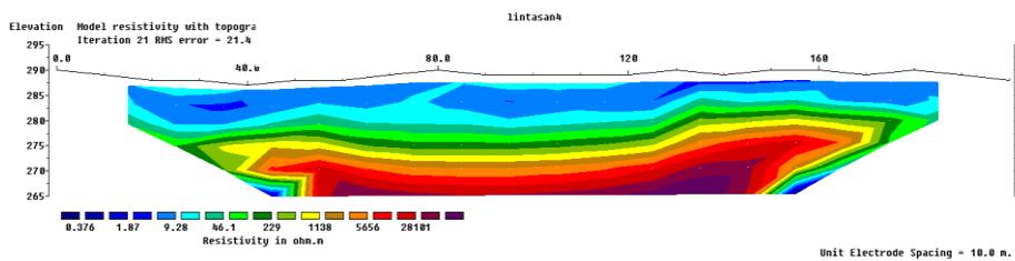
Figure 7: Subsurface resistivity 2D cross-section of line 4
