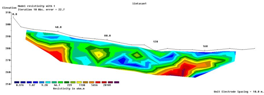
Fig 4: Subsurface resistivity 2D cross-section of line 1
