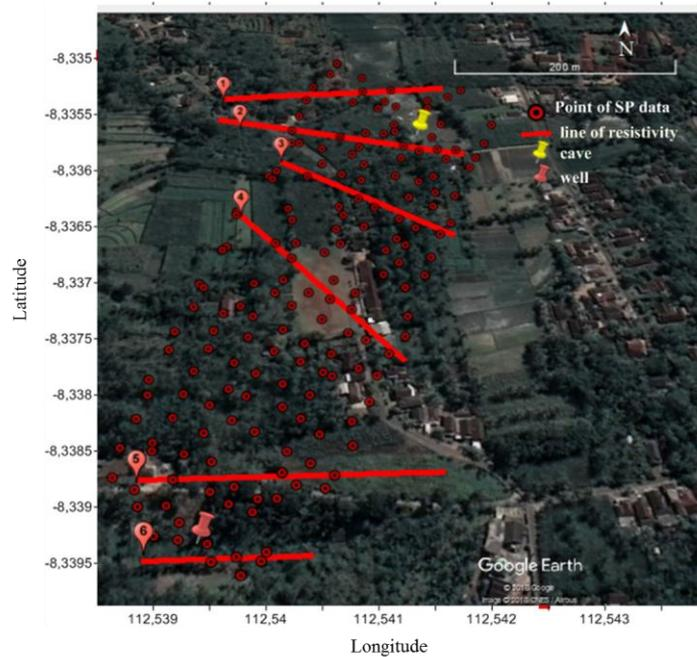
Fig 2: Geoelectrical resistivity and self-potential research survey design
