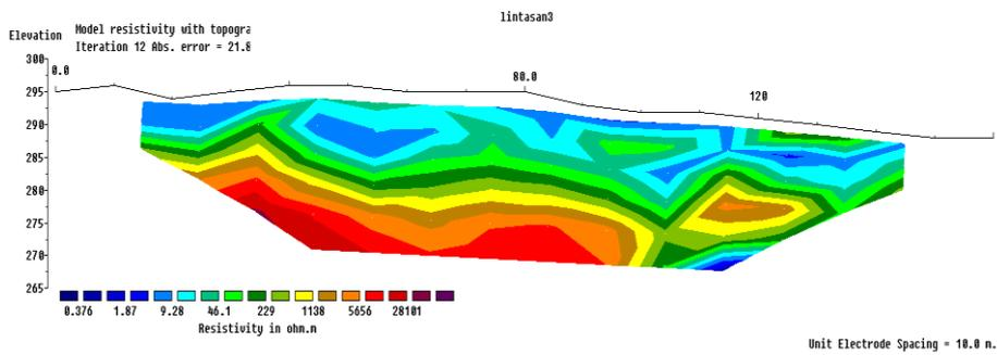
Figure 6: Subsurface resistivity 2D cross-section of line 3
