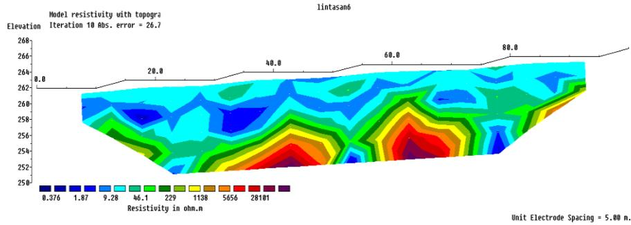
Figure 9: Subsurface resistivity 2D cross-section of line 6
