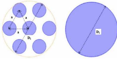
Fig.2 Cross sectional view of core region of PCF<sub>1</sub> PCF<sub>2</sub> PCF<sub>3</sub> and PCF<sub>4</sub> (Silica and BK7)
