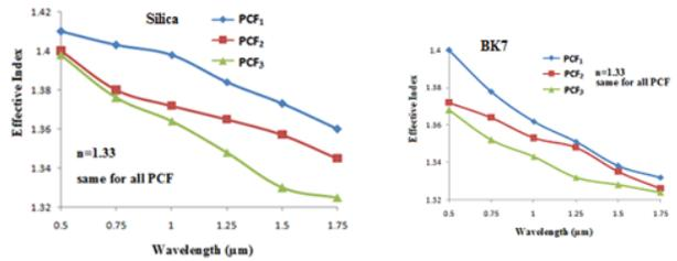
Fig.3 E effective index versus wavelength of FM X-polarization (Silica and BK7)
