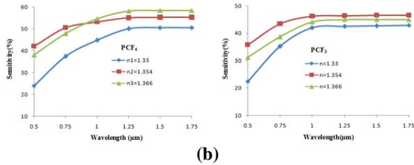
Fig.6 Relative sensitivity versus wavelength of PCF<sub>3</sub> PCF<sub>4</sub> for BK7
