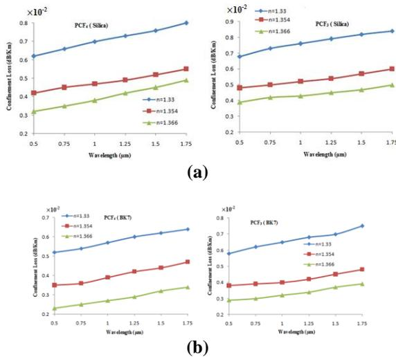
Fig.7 Confinement loss versus wavelength for PCF<sub>3</sub> and PCF<sub>4</sub> of Silica and BK7
