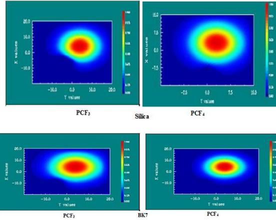
Fig.8 Modal field distribution pattern of PCF<sub>3</sub> and PCF<sub>4</sub> for X-polarized mode at an wavelength of 1.55μm (for both Silica and BK7 material)
