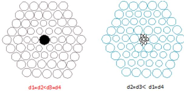
Fig.1 Cross sectional view of PCF<sub>1</sub> PCF<sub>2</sub> PCF<sub>3</sub> and PCF<sub>4</sub> (Silica and BK7)
