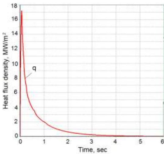
Fig. 2: Heat flux density versus time during quenching spherical steel probe 12.7 mm in diameter in 5 % water solution of NaOH at 20°C agitated with 0.914 m/s.
