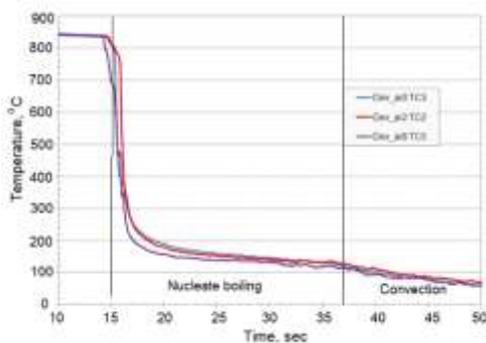
**Fig. 10:** Cooling temperature curves measured very close to surface during quenching cylindrical 2 inch probe in agitated cold water [23].
