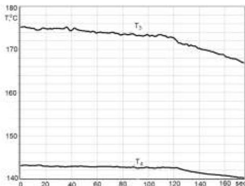
**Fig. 11:** Surface cooling curves at the distance of 220 mm and 290 mm from the end of the Probe [16]: T3 is thermocouple 3, T4 is thermocouple 4.
