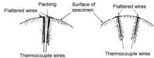
**Fig. 1:** Depiction of how thermocouples were arranged and accurately flattened to the wall of spheres and polished by French [1]
