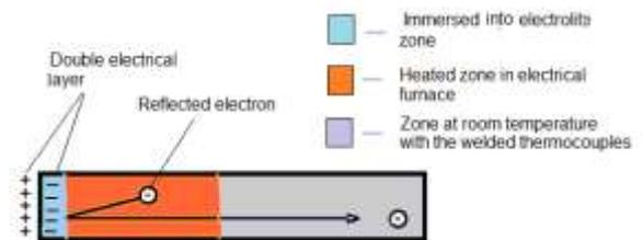
**Fig. 13:** Schematic that explains a poker effect based on laws of statistical physics [14].
