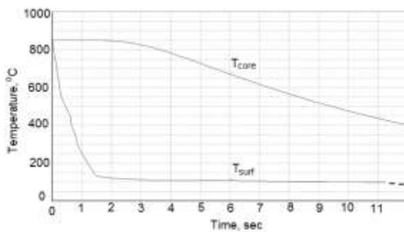
**Fig. 9:** Cooling curves obtained in Idemitsu Kosan Co., Ltd. lab, (Japan) for cylindrical specimen of 28 mm diameter and 112 mm length when quenching in water flow of 1.5 m/s at 20°C [22]
