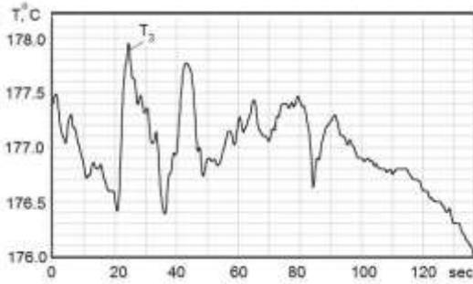
**Fig. 12:** Oscillation of the surface temperature at the distance of 220 mm (thermocouple 3) when cooling the probe in the 12% water solution of NaCl at 20°C
