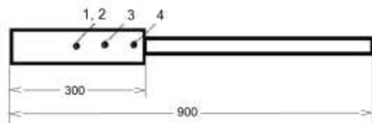
Fig 6: Probe made of carbon steel with locations of thermocouples in it [16]: 1 is a thermocouple located at the core at the distance of 150 mm from the left end of the probe, 2 is a thermocouple located on the surface of the probe at the same distance; 3 is a surface thermocouple located at the distance of 220 mm; 4 is a surface thermocouple located at the distance of 290 mm.
