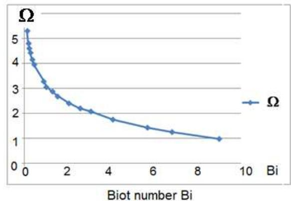
**Fig. 8:** Value  $\Omega$  versus Biot number Bi depending on size of steel part and heat transfer coefficient during convection [20].
