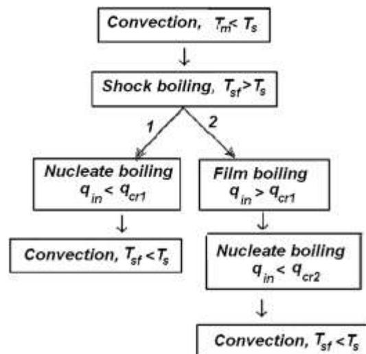
Fig. 4: The scheme of cooling process during hardening steel in cold liquid media [12].
