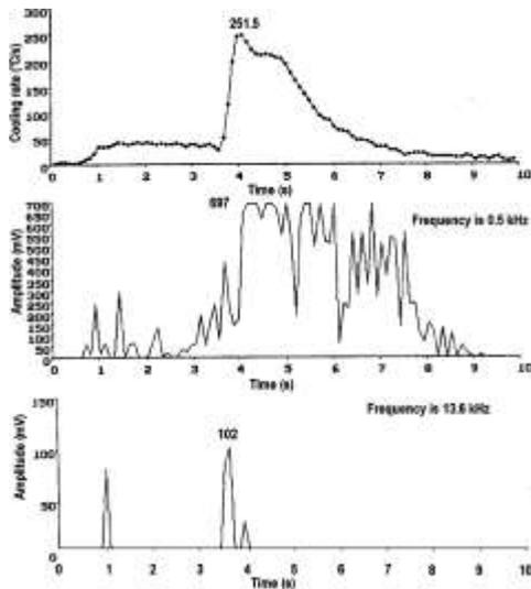
Fig. 5: Temperature–time, broadband, and narrowband quenching data [13].
