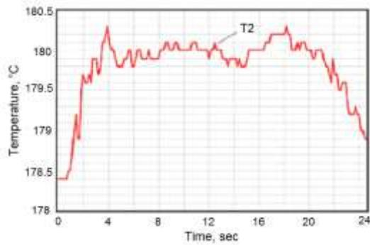
**Fig. 7:** Instant increase and oscillation of the surface temperature at a point 2 during cooling of the probe in 12% water solution of NaCl at 20°C which was immersed into solution immediately after heating (see Fig. 2)[16].
