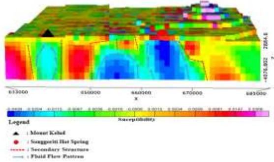
Fig. 8: Data slice on the A-A' axis for Kelud and Songgoriti geothermal system
