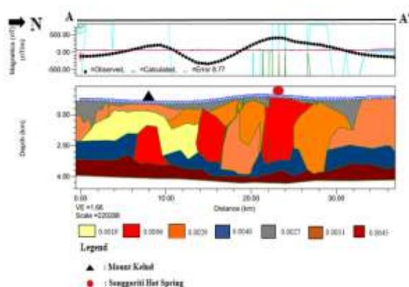
Fig. 11: Forward modeling for the magnetic anomaly in study area Kelud and Sonngoriti
