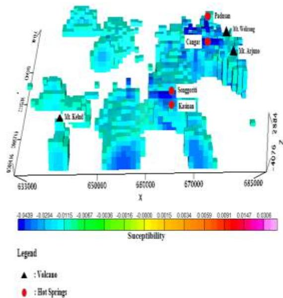
Fig. 10: The continuity between Kelud, Kasinan-Songgoriti and Arjuno-Welirang Geothermal system
