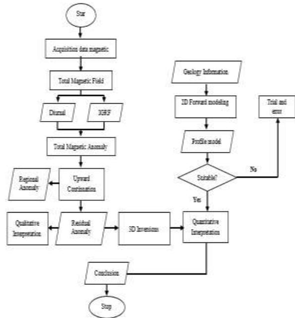
Fig. 3: Flowchart of magnetic data processing.
