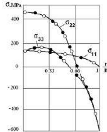
Fig. 3: Stress distribution through the section of two cylindrical specimens, one of diameter 6 mm (black data points) and the other of 60 mm (white points) at the time of the achievement of maximum compressive stresses at the surface of cylinders when Bi = 7; Fo = 0.7 [16].
