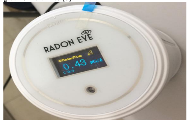
Fig 1 – Top view of Radon Eye RD200 ionization chamber used for monitoring radon gas [6]
