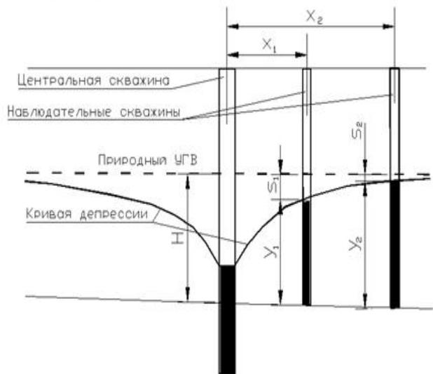
**Fig. 1. Draw-down funnel for a shallow well (or well)**
