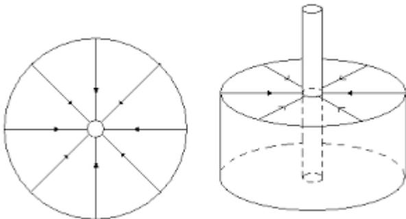
**Fig. 2. Scheme of radial filtration of water from the reservoir to the well.**
