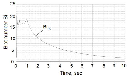
**Fig. 6: Real Biot number versus time during quenching cylindrical probe 20 mm diameter in water 20°C under pressure 1 MPa.**
