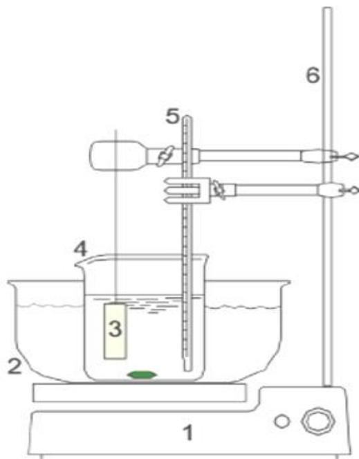
Fig. 1 Experimental setup of chemical bath deposition technique [10] (Yi-Cheng et al., 2014)
