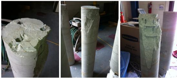
Specimen 1, Specimen 2, Specimen 3 Figure 6: Failure in Shaft Specimens after Testing
