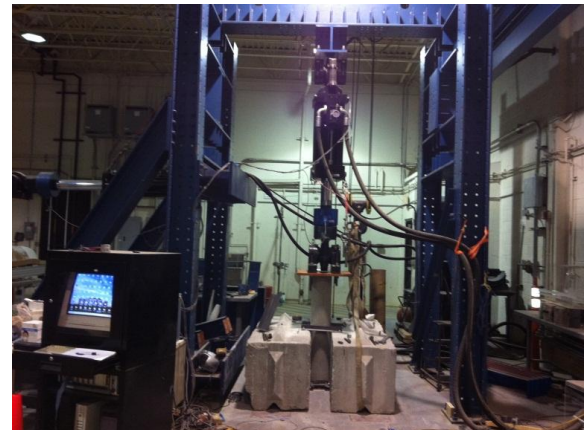
Figure 4: Hydraulic Actuator Machine Used for the Tests
