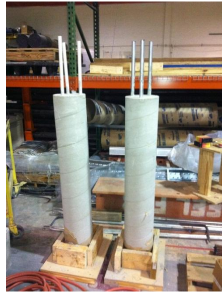
Figure 2. Specimen 1 with PVC Tube and Specimen 2 with Galvanized Tube
