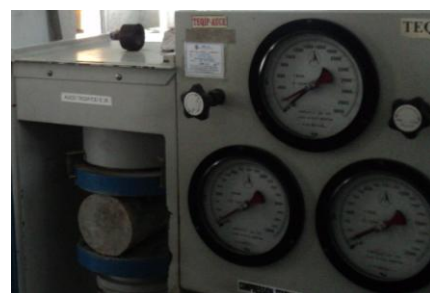
Figure 5 Split Tensile Strength testing
