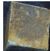
Figure 3 Acid effected concrete cubes
