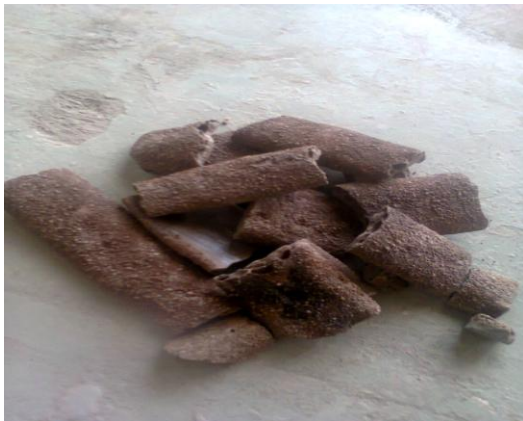
Fig. 1 Fused submerged arc welding flux waste
