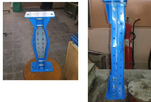
Fig. 19 The failure mode of a single column compression loading test
