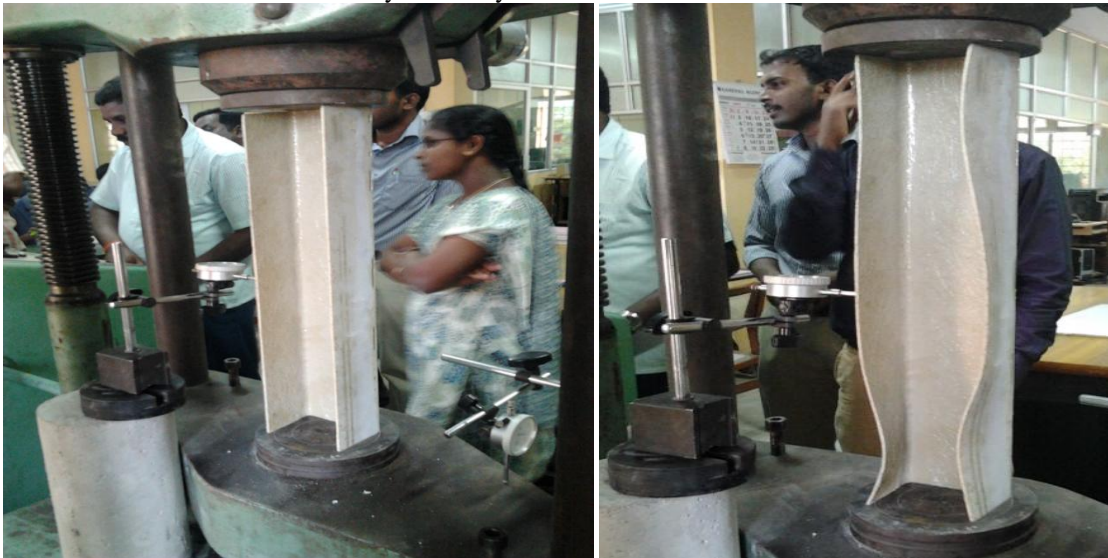
Fig 2. Specimen EFC 100-75-3 -500 reaches the ultimate load of 32 kN by UTM test.
