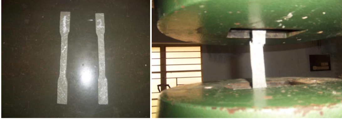
Fig 1 Failure of Coupon Specimen (Epoxy Resin)
