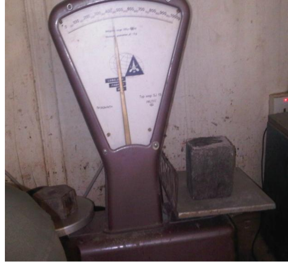
Figure 3.2: Weighing of Hardened Concrete Cube
