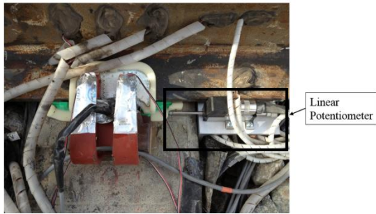
Figure 11. Linear Potentiometer Placement in the Field Experimentation at TTC
