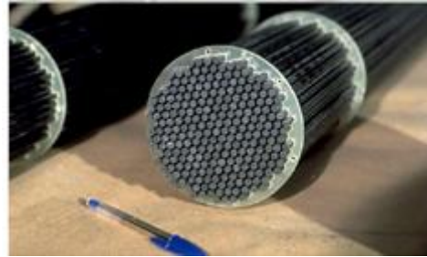
Figure 3: CFRP cable consisting of 241 wire.”SOURCE: Meier[4]”
