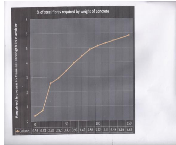
Figure 5 Percentage of steel fibres w.r.t desired increase in flexural strength
