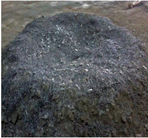
Fig. 1 CSF and WWA Added Mix before Casting
