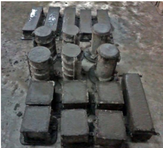
Fig. 2 Moulds filled with Concrete before Curing
