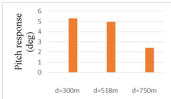
Fig. 6 Comparison of Pitch Response Hs=16m
