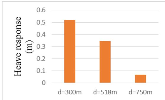
Fig. 5 Comparison of Heave Response Hs=16m
