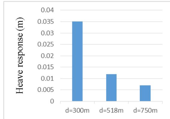
Fig. 8 Comparison of Heave Response Without Wave
