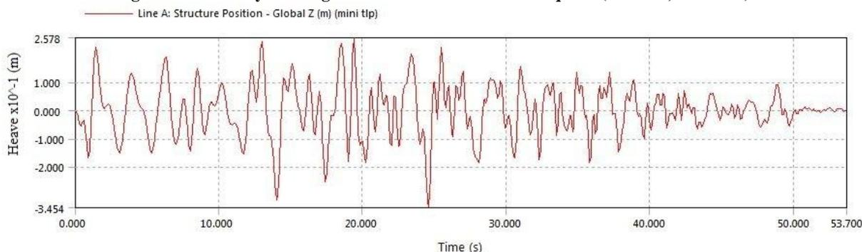
Fig. 12 Time History of Heave Under the Presence of Earthquake (Hs=16m, Tz=20sec)
