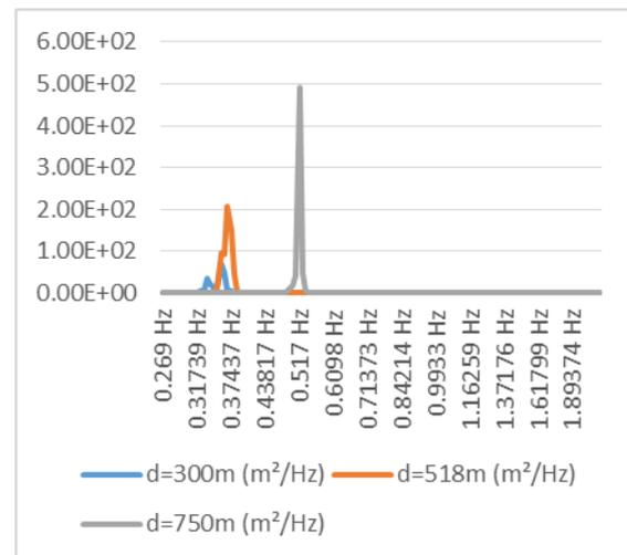
Fig. 10 Spectral Distribution for Surge (Hs=16m)
