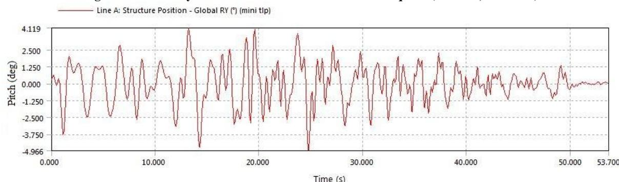
Fig. 13 Time History of Pitch Under the Presence of Earthquake (Hs=16m, Tz=20sec)
