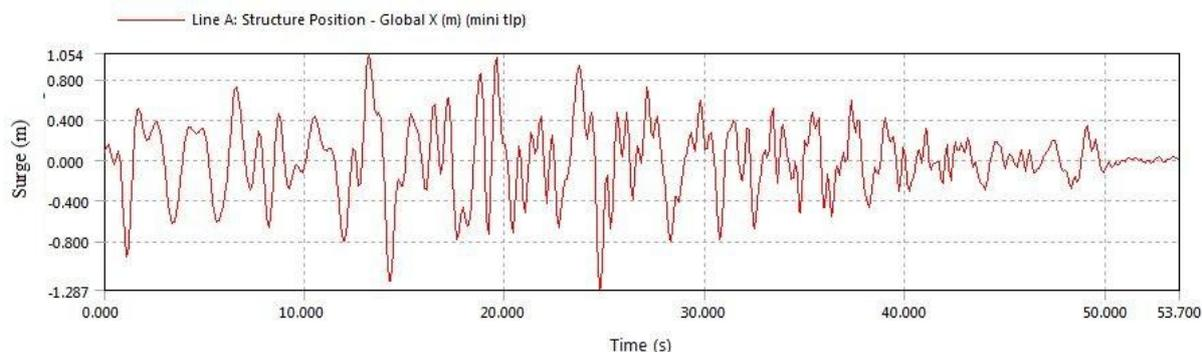
Fig. 11 Time history for Surge Under the Presence of Earthquake (Hs=16m, Tz=20sec)
