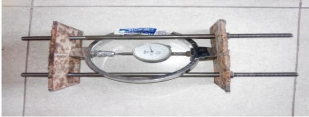
Fig.1 Arrangement of Proving Ring With Calibration Rod
