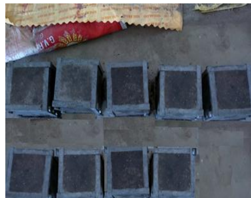
Fig. 4 Cubes After Casting
