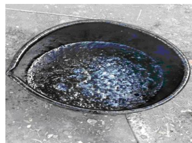
Fig. 3: Foam Modified Bitumen
