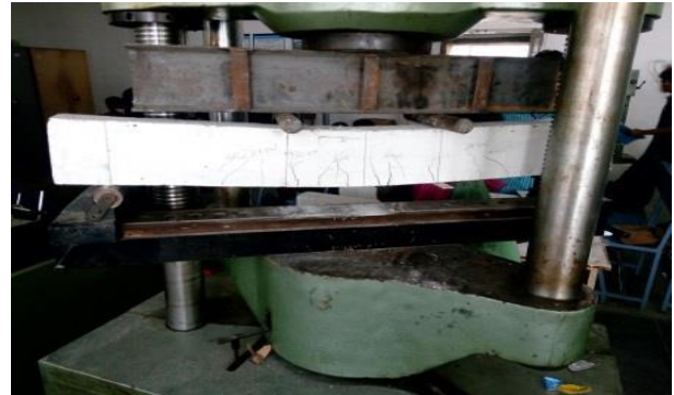
Fig 5. Three Point Loading Flexural Test of RC Beam
