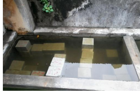
Curing Of Cubes
