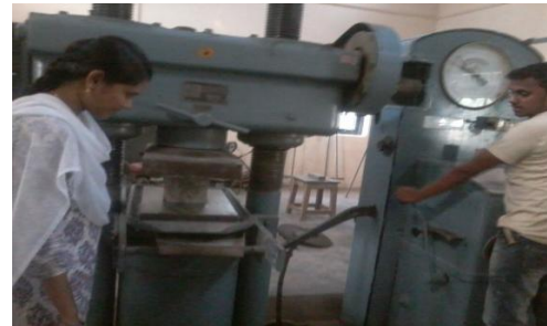
Testing of cubes
