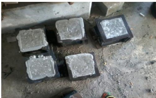
Casting of cubes
