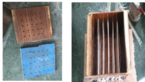
Fig :7 Mould Used for Casting Translucent Concrete
