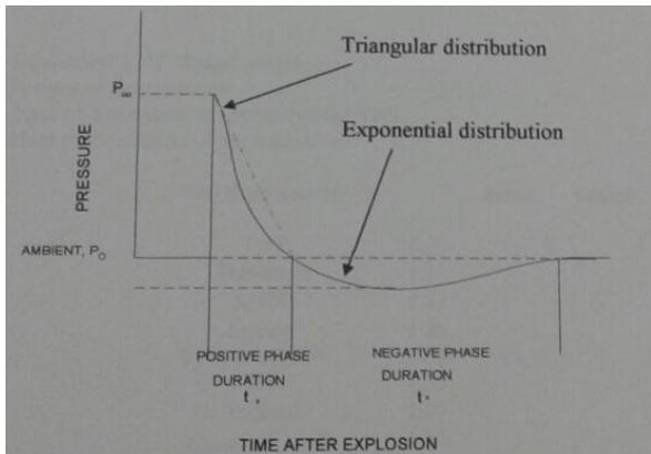
**Fig. 1 Exponential and Triangular Distribution of Pressure due to Blast Load**
