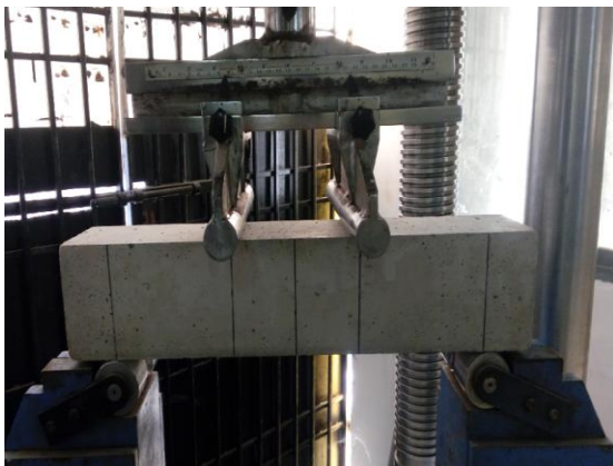
Fig.5 Flexural Strength testing
