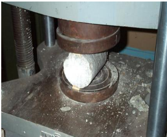
Fig.3 Split Tensile testing
