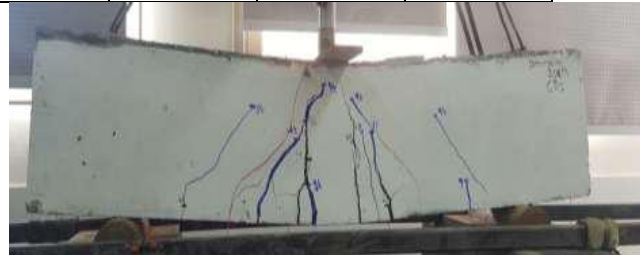
Fig. 4 Failure Cracks for Control Beam B1
