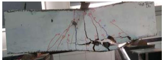
Fig.5 Failure Cracks for Strengthened Control Beam B2
