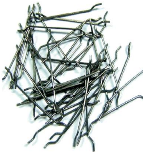
a) Hooked end steel fibers
