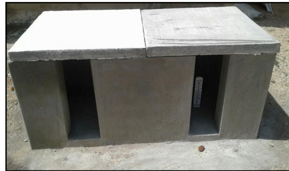
Figure 4: Model room with RC slab
