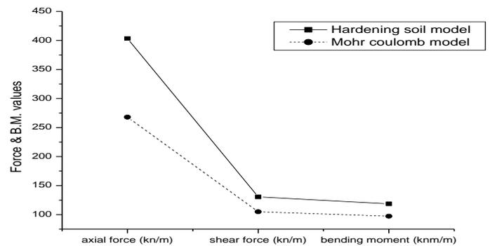
Fig 11: S.F, B.M, & Axial Force Comparison Between Both Models.
