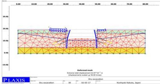
**Fig 3: Deformed mesh final stage.**
