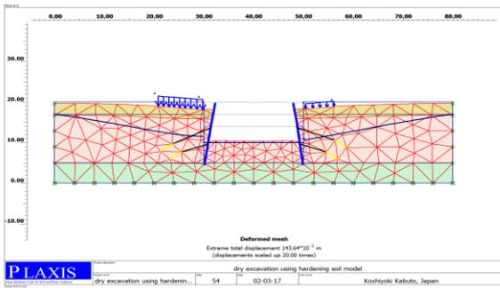
Fig 7: Deformed mesh final stage
