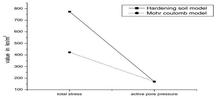
Fig 12: Total Stress & Active Pore Pressure Comparison Between Both Models.
