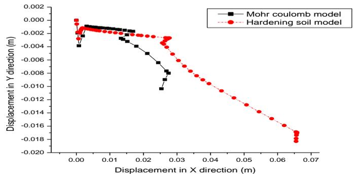
Fig 13: Displacement in X & Y Direction.
