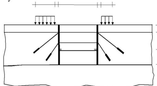
Fig 1: Excavation Diagram With tie Back Walls
