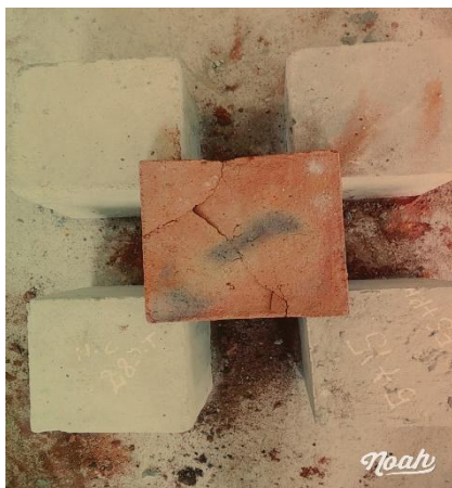
Fig 5: Cracks on tile after failure load
