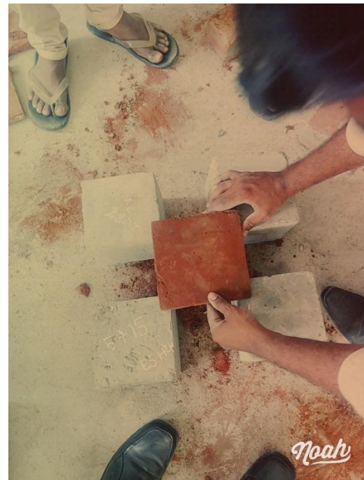
Fig 2: Placing of Tile on Concrete Cube Base
