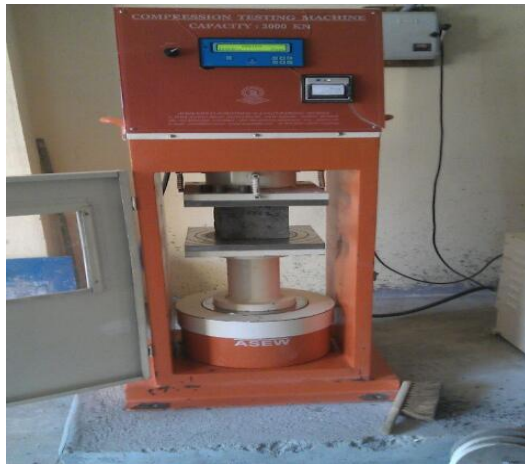
Fig-1 Cube Compression Test
