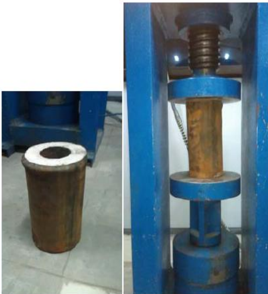
Fig. 2 Concentrically Welded Steel Tubes
