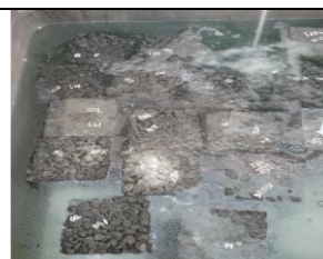
Pic 3: Cubes and Cylinders for 7day and 28 days
