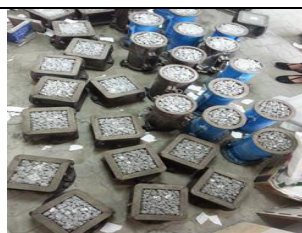
Pic 2: Casting Cubes and Cylinders of Porous Concrete
