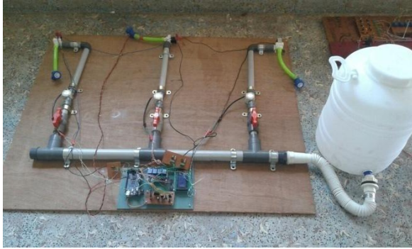
Fig. 4. Automated Model For Three House Units
