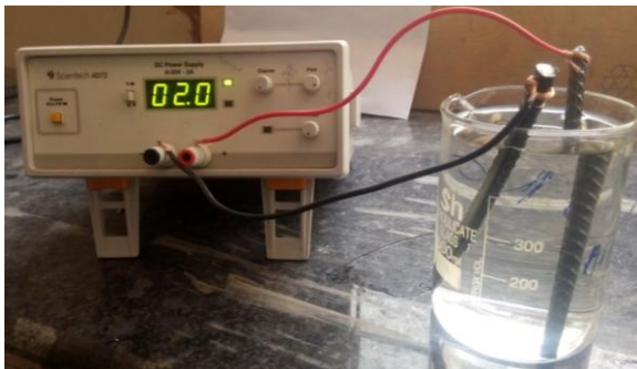
Fig. 5 No Rust Formation in Coal Tar Epoxy Coated Rebar
