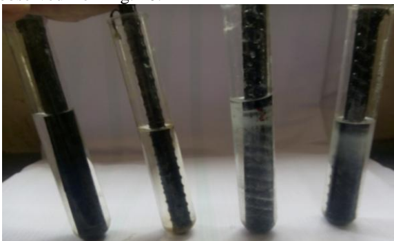
Fig. 10 Discolouration in Coated Rebars at the End of 45 Days Test Period
