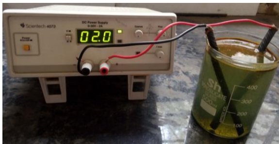
Fig. 4 Rust Formation in Uncoated Rebar
