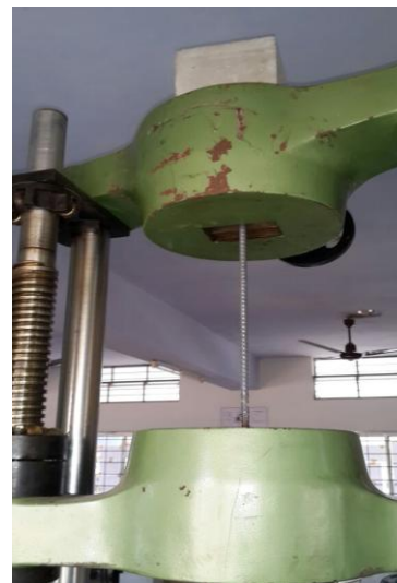
Fig. 3 Pull Out Test Setup
