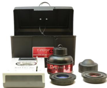
Fig. 5: Image Showing the Equipment Used During the Study, the Elements that Compose it are the Meter, a Tamper-Resistant Case, a Short-Time Camera, A Long-Time Camera, a Short (Blue) And A Long (Red) Electrete.
