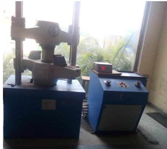
Fig 4: Compressive Strength Testing of Cubes
