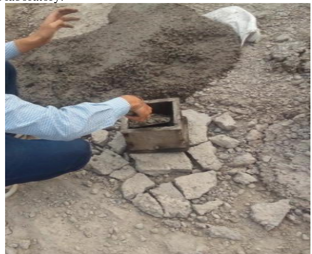
Fig 1: Mixing of Multiblended Concrete
