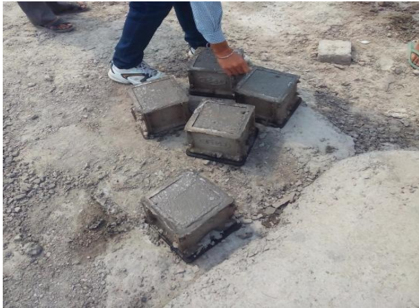
Fig 2: Casting of Cubes
