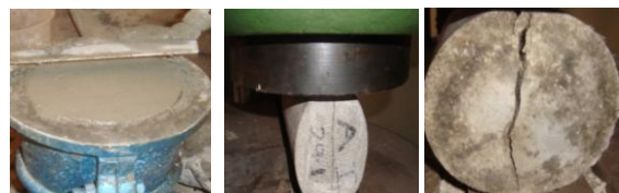
Fig.2 Casting and Testing of Cylinder
