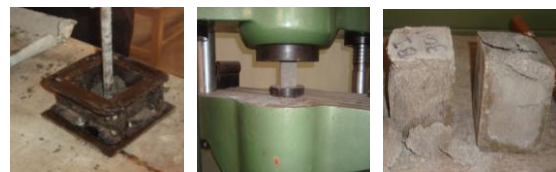
Fig.1 Casting and Testing of Cube
