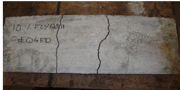
Fig.14 Failure of Geogrid Mesh Panel
