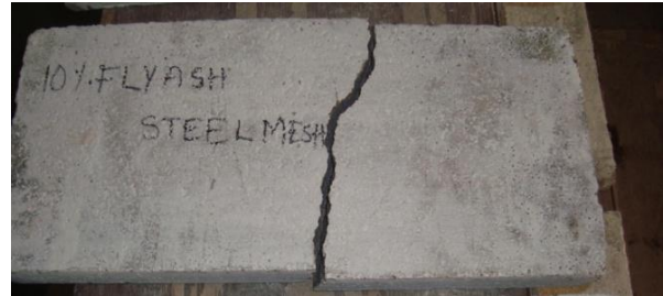
Fig.13 Failure of Steel Wire Mesh Panel
